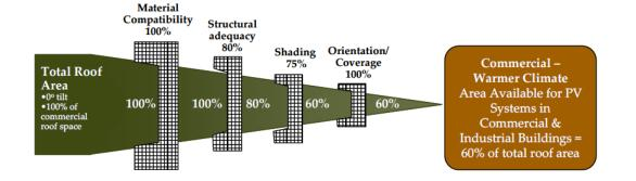
60%-65% of the commercial rooftop area is suitable for solar PV installation.
