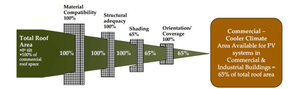
Figure 6. PV access factor for commercial buildings in cooler climates
